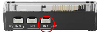
Plug light sensor into IN 1
