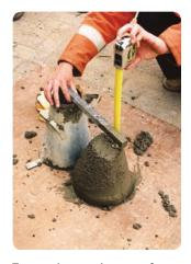
To test the consistency of concrete, inspectors perform a slump test by forming a cone of concrete and measuring how much it slumps due to gravity.
